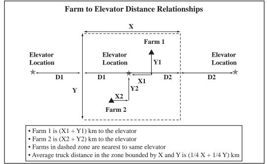
Figure 1: Farm to Elevator Trucking Distance on a North-South / East-West Grid
