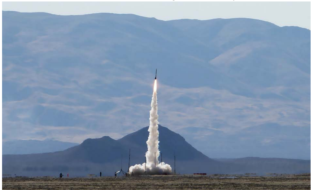
Liftoff of an ARLISS rocket to launch a small CanSat test unit at 12,000 feet.
