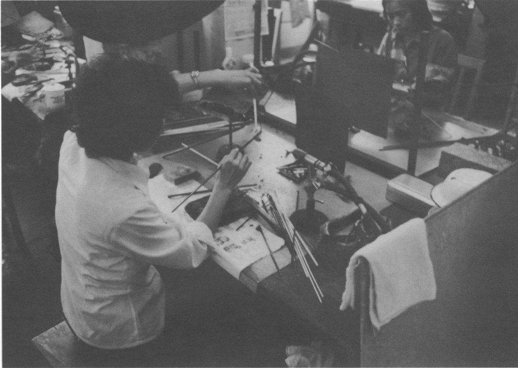
Figure 3. The use of tweezers to manipulate a glass object at the Beijing Glass Ware Factory (photo by R. Sprague).
