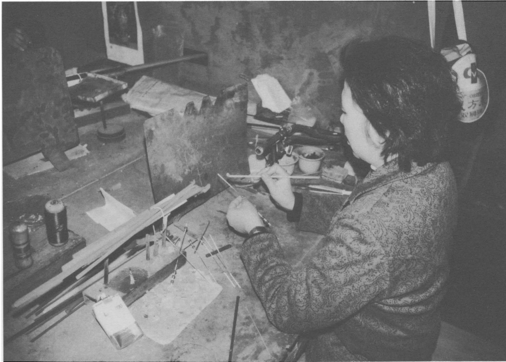
Figure 6. Zhang Yuxia of the Beijing Glass Ware Factory making wound beads (photo by R. Sprague).
