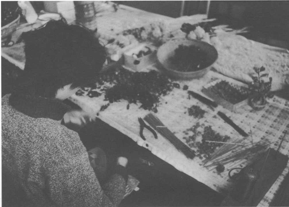
Figure 5. Worker in the Beijing Glass Ware Factory making jade trees from glass components (photo by R. Sprague).
