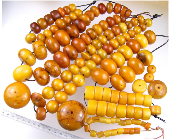
Figure 1. Beads of phenol-formaldehyde thermosetting resins (PFs) from the African trade. The large bead at bottom center is 52.9 mm in diameter (metric scale) (all images by the author unless otherwise noted).
