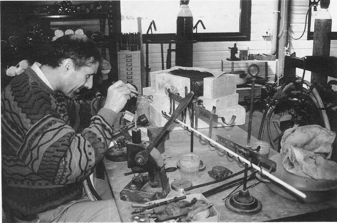
Figure 12. Gérard Alexanian making imitation granite beads. These are mold-pressed beads made using original Rousselet mixed crushed glass.
